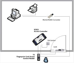
Single door separate type access control solution
