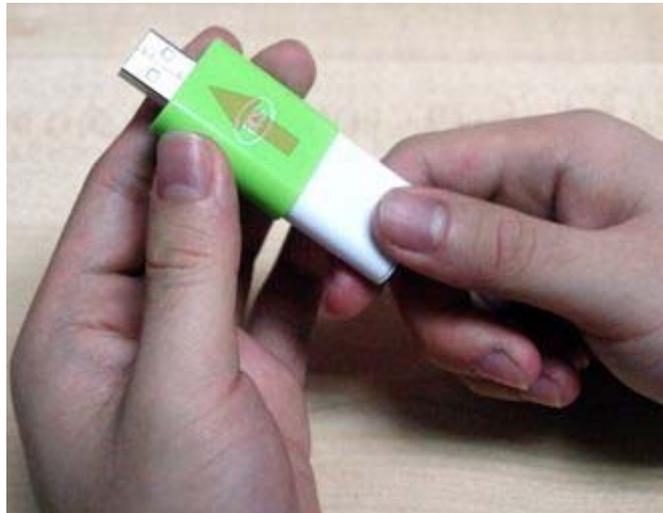
3. Place your thumb on the cover of the SIM-sized smart card slot and push up.
