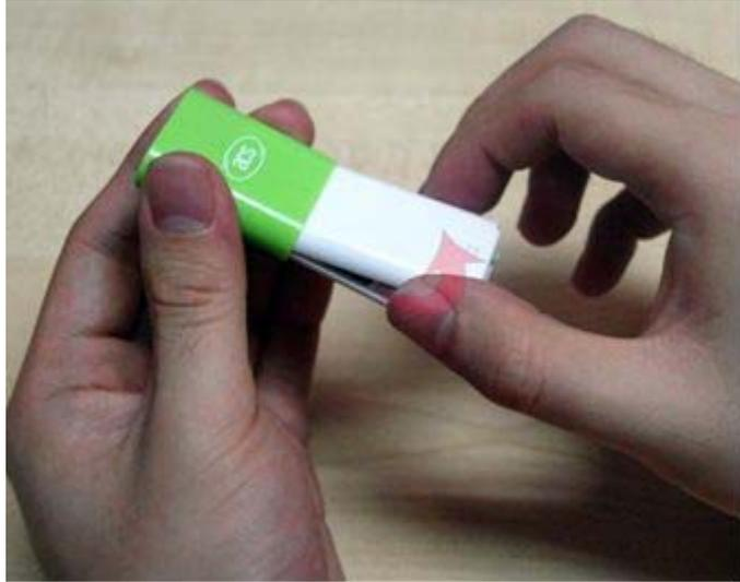
5. Remove the cover to reveal the SIM-sized card and MicroSD slot.
