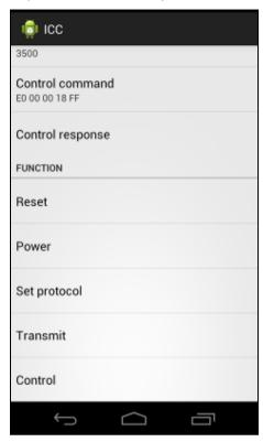
5. Under **Function**, tap **Transmit** to execute the APDU command. The reponse will be displayed under Response APDU.
