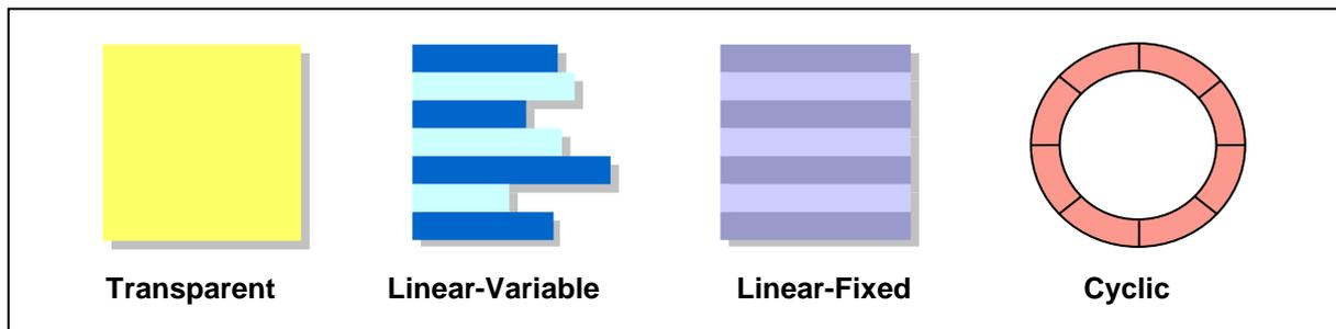
**Figure 3:** Structures of Elementary Files According to ISO 7816-4
