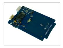
The ACM1281U-C7 USB Contactless Reader Module with SAM Slot, running on the 13.56 MHz frequency, was designed for fast and easy integration to embedded systems. It supports ISO 14443 Parts 1-4 Type A and B cards, and MIFARE Classic® series.
