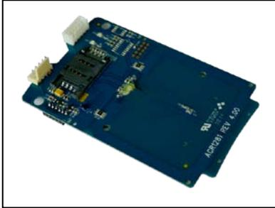
The ACM1281 is a Contactless Reader Module with SAM Slot designed based on the 13.56 MHz technology. It supports ISO 14443 Parts 1-4 Type A and B cards, and MIFARE® Classic series with a card reading distance of up to 50 mm (depending on tag type).
