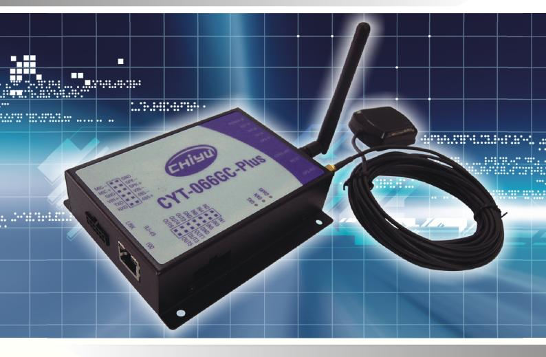
CYT-066GC-Plus enable Chiyu Web based door controller transfer and receive data via GPRS. Support for web management & firmware upgrade. Easy Network connection not only protects your exited device but also has more extendable network environment for further using. Thru CYT-066GC-Plus, you can control all devices simultaneously. Therefore, CYT-066GC-Plus is very suitable for some places will are hard for wiring connection.
