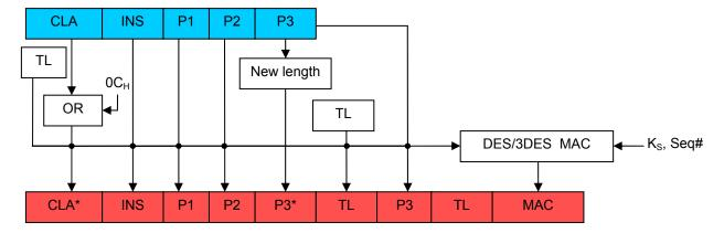
The following figure shows the command transformation of a command with data (ISO-IN) to a secure messaging APDU command:
