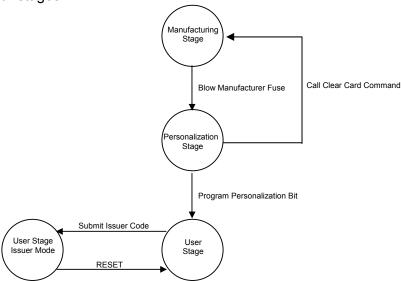
The actual chip life cycle stage is determined by the card operating system immediately after a reset. The life cycle stage does not change during the operation of the card. Clear card command can be issued in the personalization stage and manufacture state to clear the card of all data. However, this command will not be able to be used after User Stage.
