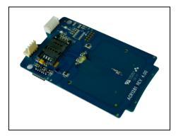
The ACM1281S-C7 Serial Contactless Reader Module with SAM Slot is designed based on the 13.56 MHz technology. It supports ISO 14443 Parts 1-4 Type A and B cards, and MIFARE Classic® series with a card reading distance of up to 50 mm (depending on tag type).
